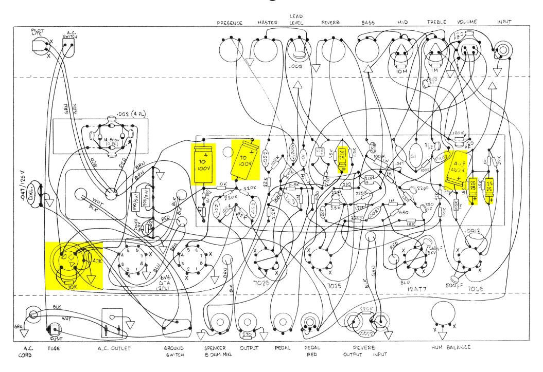
Fender Princeton Reverb II Amplifier Wiring Diagram
